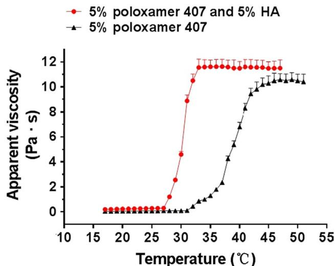
**FIGURE 2** Temperature-viscosity Curve of hydrogel. Apparent viscosity ( $\eta$ ) of HA-POL hydrogel or POL 407 was examined at different temperatures (t)
