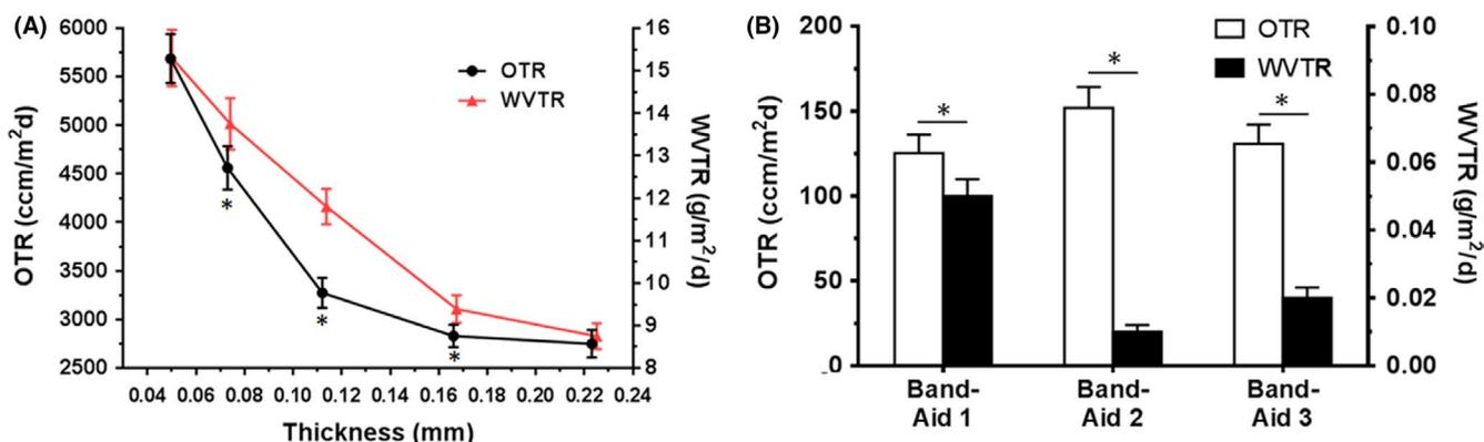
**FIGURE 6** WVTR and OTR curve of films formed by HA-POL gel with different thickness. A, HA-POL hydrogel was used to form a film. The WVTR and OTR of films formed by HA-POL hydrogel with different thickness was examined. B, The WVTR and OTR of three kinds of Band-Aid with different thickness (Band-Aid 1: 1.5mm; Band-Aid 2: 0.8mm; and Band-Aid 3: 1.0mm) was examined as control. \* $P < 0.05$
