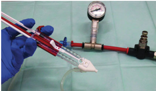
FIG. 1. Spray setup with pressure regulator and -gauge (at the top), spraying nozzle (front), and syringe holder with syringes (left).
