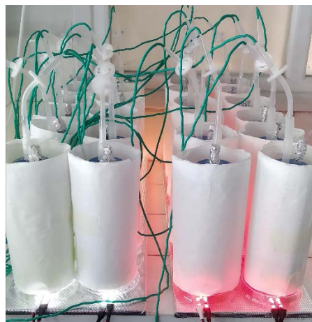
Figure A1. Experimental configuration for growing A. protothecoides with monochromatic illumination by LEDs in 500 mL flasks aerated with sterilized air.
