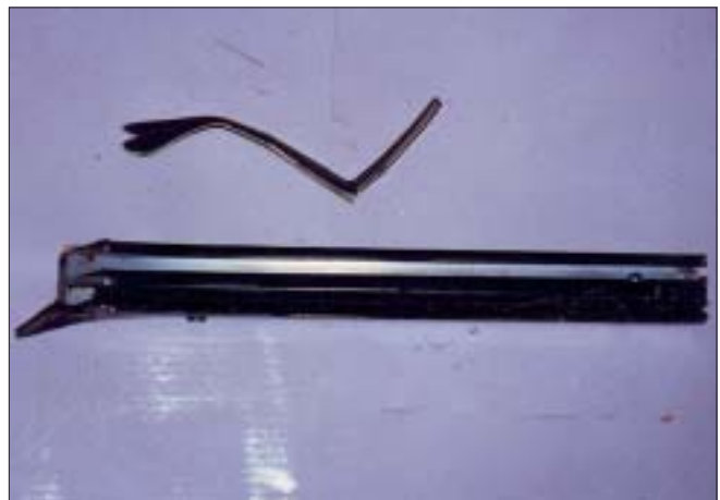
Figure 2: Photograph showing the removed fencing (lower) and spectacle (upper) sidebar
