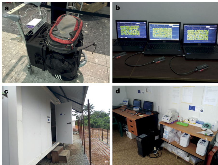
Figure 7. Portable genome sequencing for Ebola surveillance in Guinea. The system consisted of three MinION instruments, four laptops, a thermocycler for PCR, and other tools. Panel (a) shows that the authors used aircraft baggage to carry all instruments, reagents and disposable consumables. Panel (b) shows that the authors initially established the genomic surveillance laboratory in Donka Hospital, Conakry. Panel (c) is used to indicate that they later moved the laboratory to a dedicated sequencing laboratory in Coyah prefecture. Panel (d) shows an image of the room inside this laboratory where they separated the sequencing instruments (left side) from the PCR bench (right side). Power to the thermocycler was provided by an un-interruptable power supply, which can be observed in the middle of the room. (Photos were taken by Josh Quick and Sophie Duraffour.) Reprint from [153].
