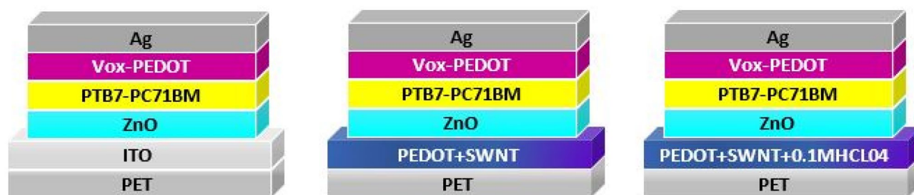
Figure 1. Schematic device structure based on PET/PEDOT-SWCNT, PET/PEDOT-SWCNT + (0.1 M) \text{HClO}_4 and ITO cathodes.
