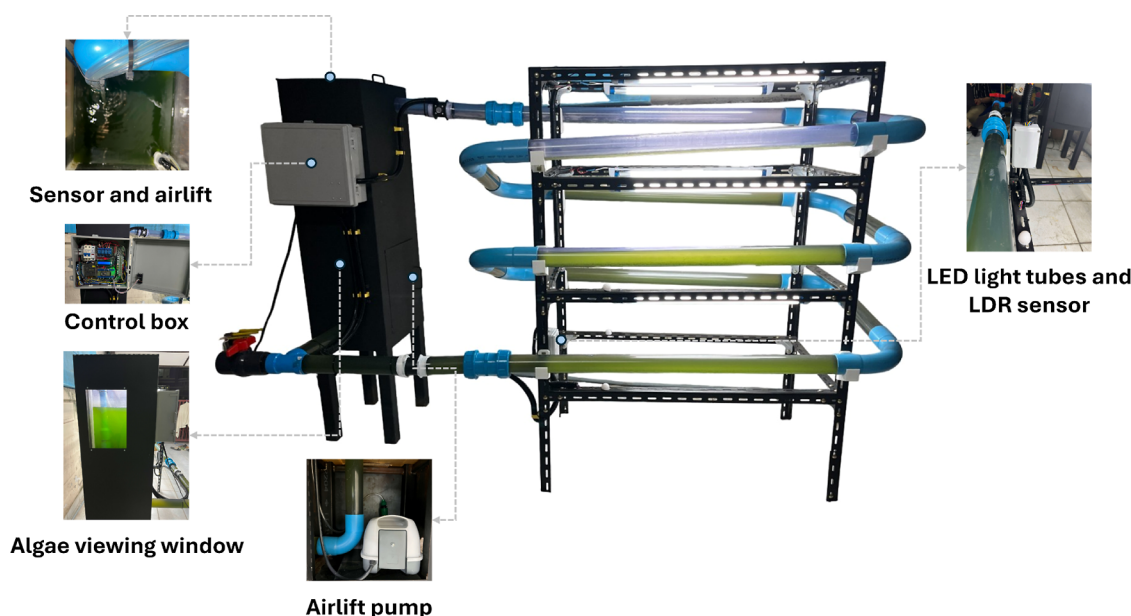
Figure 1. Schematic diagram and components of the closed tubular PBR system for Chlorella sp. cultivation.
