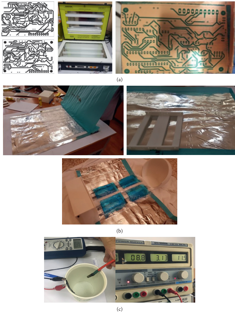
FIGURE 5: Demonstration of the real prototype's implementation and testing. (a) PCB process. (b) Sewer process. (c) The laboratory setup utilized for testing the warming system component's of the Handy incubator.
