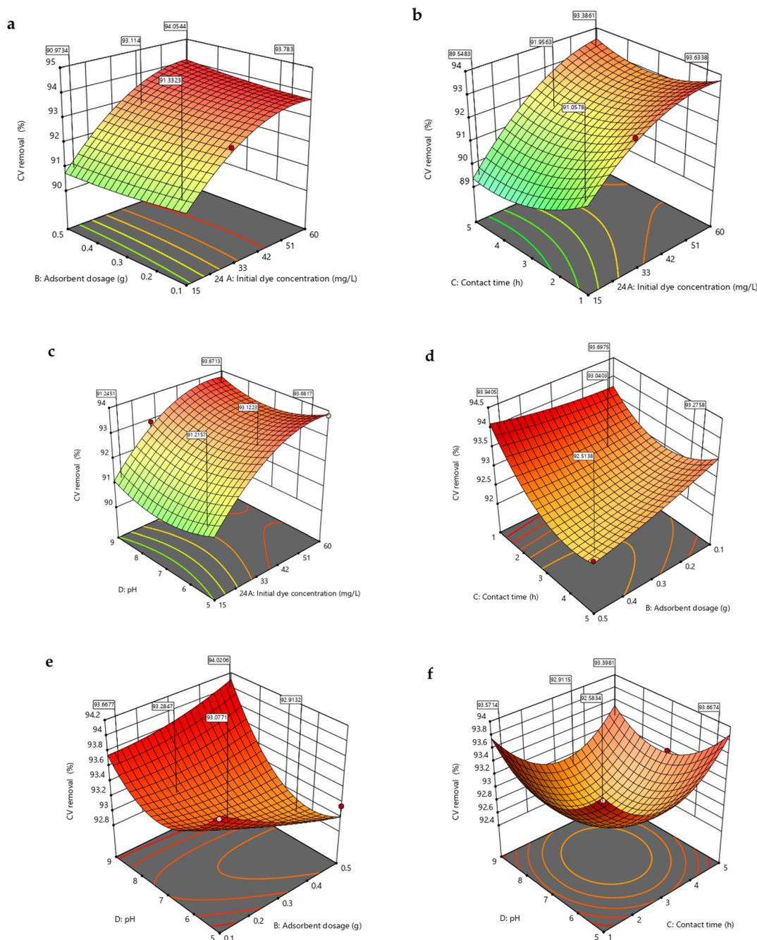
Fig. 6 RSM 3-D plots for CV removal (60 mg L<sup>-1</sup> initial dye conc., 1 h contact time, 9 pH and 0.1 g adsorbent dosage) (a) adsorbent dose and initial dye concentration (b) contact time and initial dye concentration (c) pH and initial dye concentration (d) contact time and adsorbent dose (e) adsorbent dose and pH (f) pH and contact time.
