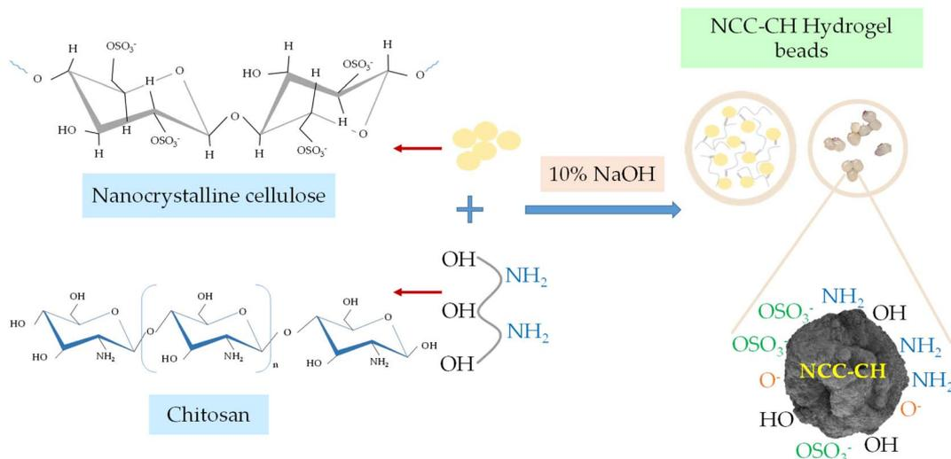
Fig. 1 Preparation of Nanocrystalline cellulose–chitosan hydrogel beads.
