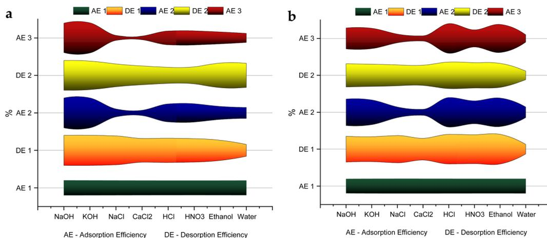
Fig. 10 Variation in adsorption and desorption efficiency of NCC-CH under different desorbents (a) CV and (b) MB.
