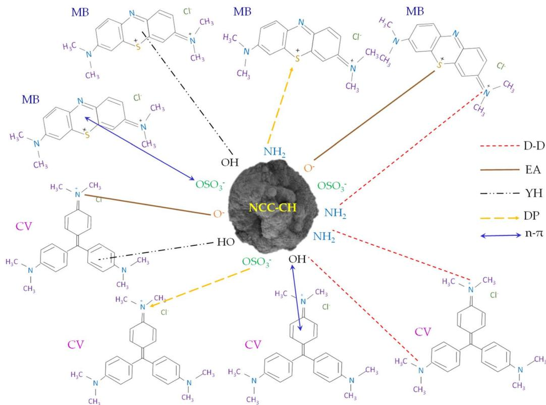
\*D-D - Dipole-dipole Hydrogen bonding; EA – Electrostatic attraction; YH – Yoshida H-bonding; DP – Dipolar bond and  $n-\pi$  -  $n-\pi$  stacking interaction
