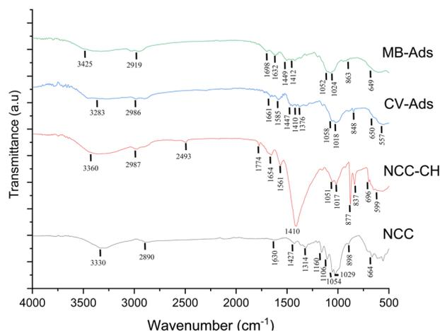
Fig. 5 FTIR analysis of NCC and NCC-CH hydrogel beads before and after dye adsorption.
