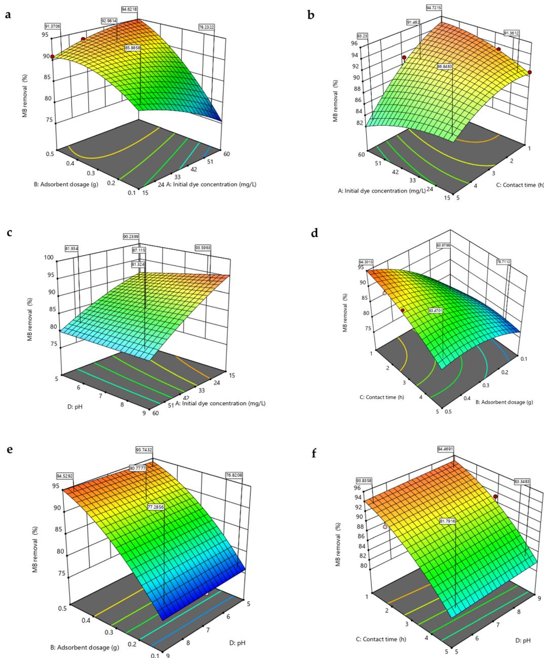
Fig. 7 RSM 3-D plots for MB removal (60 mg L<sup>-1</sup> initial dye conc., 1 h contact time, 9 pH and 0.5 g adsorbent dosage) (a) adsorbent dose and initial dye concentration (b) contact time and initial dye concentration (c) pH and initial dye concentration (d) contact time and adsorbent dose (e) adsorbent dose and pH (f) pH and contact time.
