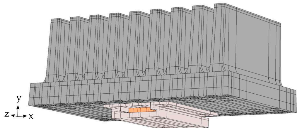
Figure 8. Geometry of the numerical model. Dark grey—heat sink, light grey—aluminum body of the heater, orange—active heater domain.
