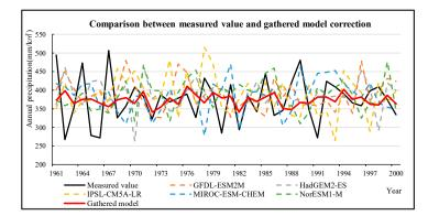
**Figure 7.** Comparison between the measured value and the gathered model correction (annual precipitation from 1961 to 2000). The red line is the gathered model value, which was closer to the measured value (black line) compared to the different model values (colored lines).
