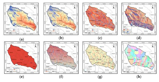
**Figure 5.** Sub-watershed and Slope-confluence calculation order formation processes ((**a**) Digital Elevation Model (DEM); (**b**) revised DEM; (**c**) slope; (**d**) flow direction; (**e**) flow accumulation; (**f**) calculation order of slope confluence; (**g**) river code; (**h**) sub-basin).
