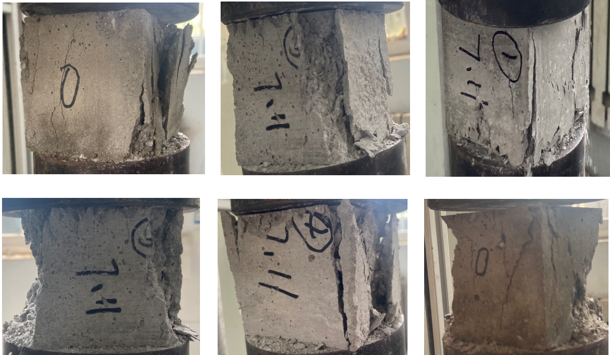
Figure 10. Different ratios of failure modes.
