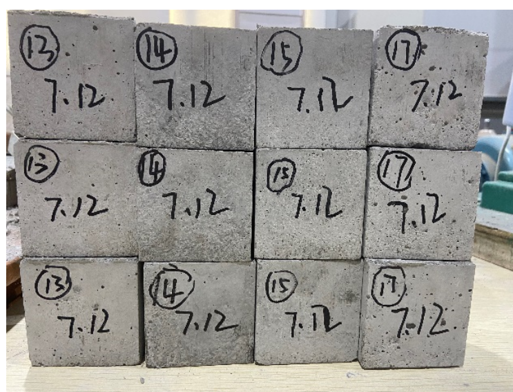
Figure 1. Specimen of microconcrete.
