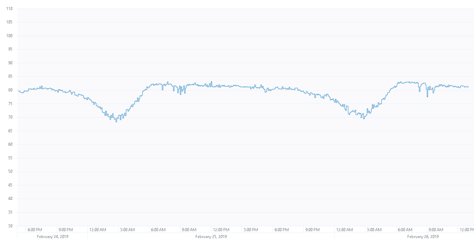
Figure 3. Example of two-day L_{Aeq300} curve of sensor hb148. The vertical axis is the measured L_{Aeq300} , in dB.
