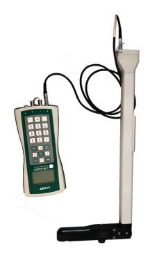
Figure 4. LAI-2200C plant canopy analyzer.
