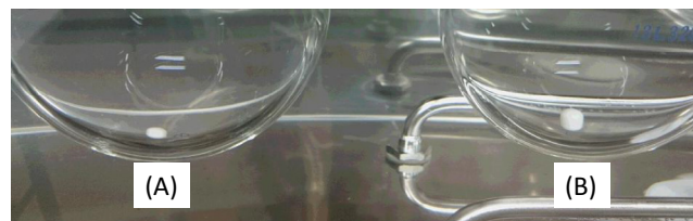
Fig. 2 – A picture of remaining tablet after 7h dissolution test in test medium (pH 1.2) using USP apparatus 2 (200 rpm). (A) Rp. 1: HPMCAS-based matrix tablet, (B) Rp. 3: HPMCAS/HPC ER matrix tablet.
