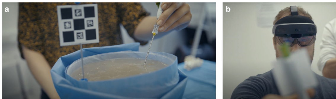
Fig. 1 a A ChArUco marker in a phantom. b A user wearing the HoloLens 2™
