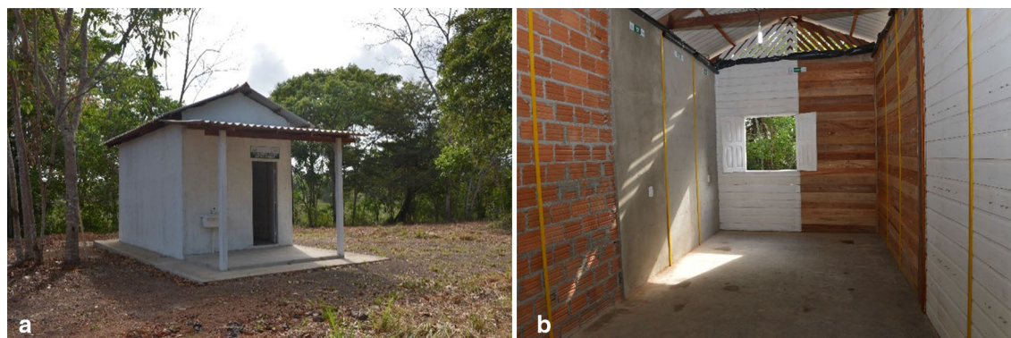
Fig. 2 Test house external view. a Frontal and lateral view of the external plastered cement surfaces painted with acrylic paint. b The view of the side surfaces of unplastered cement (CP2) and plastered cement (CP1) divided into strips for the application of insecticides; view of the back wall (control) consisting of a painted wooden wall (WP1) and an unpainted wooden wall (WP2); a corrugated fiber cement roof and a bare concrete floor
