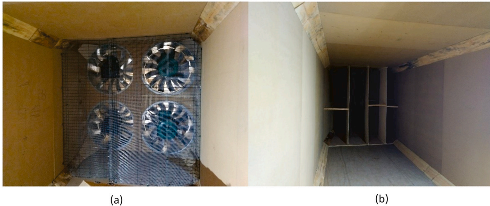
Fig. 5. View of the secondary chamber. (a) Suction of the fans. (b) Deflectors.
