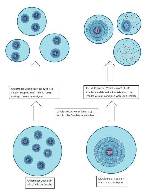
**Figure 5.** Liposome disruption during exposure to nebulization. Reprinted with permission from [30]. Copyright 2013 Future Science.
