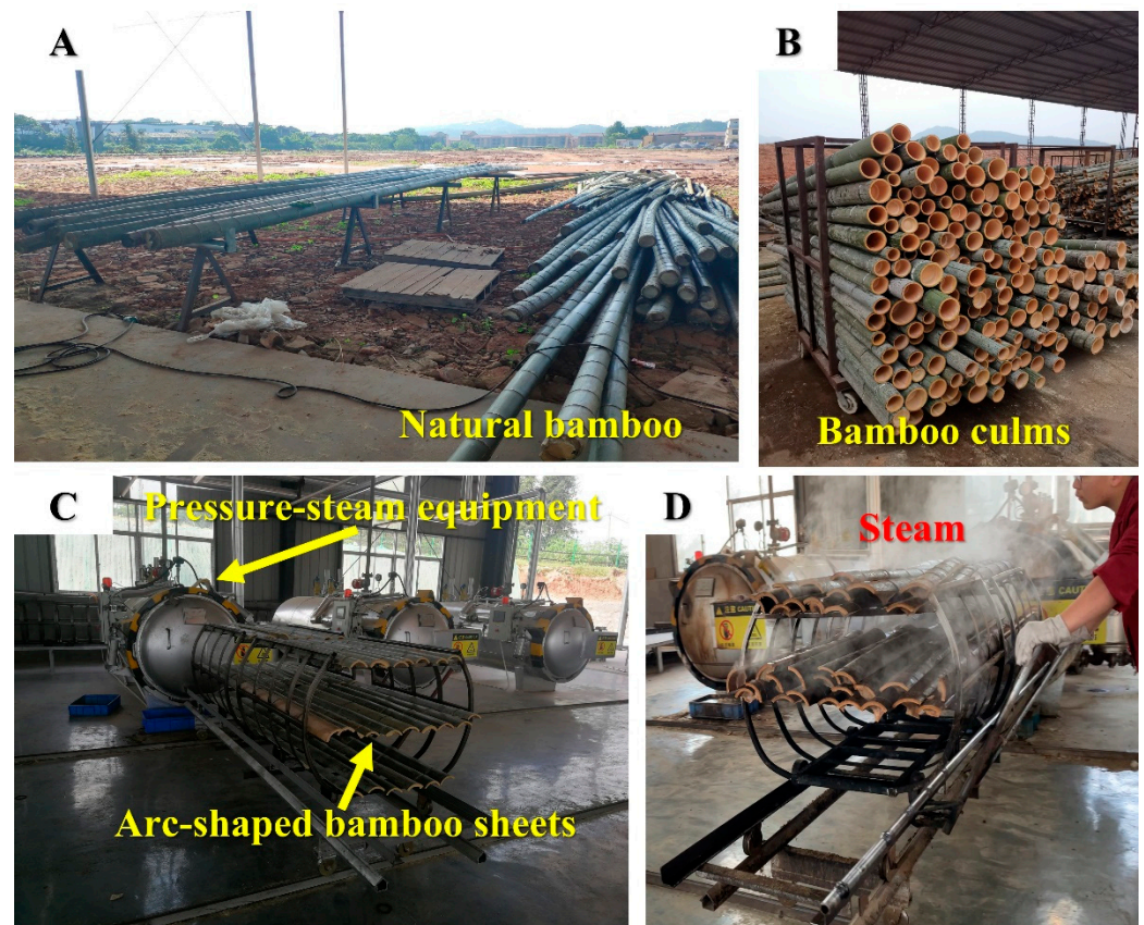
Figure 1. Heat treatment process of bamboo: (A) Natural Bamboo in factory; (B) Bamboo culms; (C) Pressure-steam equipment and arc-shaped bamboo sheets; (D) the bamboo sample after saturated-steam heat treatment.
