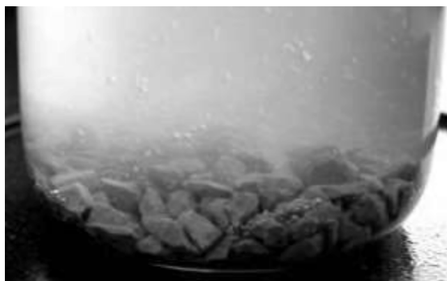
Fig. 6. Isolation of air bubbles from clinoptilolite particles (2.5–3.0 mm) under the action of ultrasonic irradiation (ultrasonic power as 10.2 W (0.102 W/mL); \text{C}(\text{AgNO}_3) = 0.01 \text{ M} ; temperature as 25^\circ\text{C} ).
