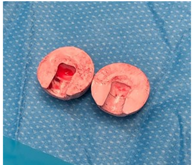
Figure 1. Replacement BIOLOX delta ceramic femoral head, split into two large pieces without fragmentation after impaction onto the native femoral head.
