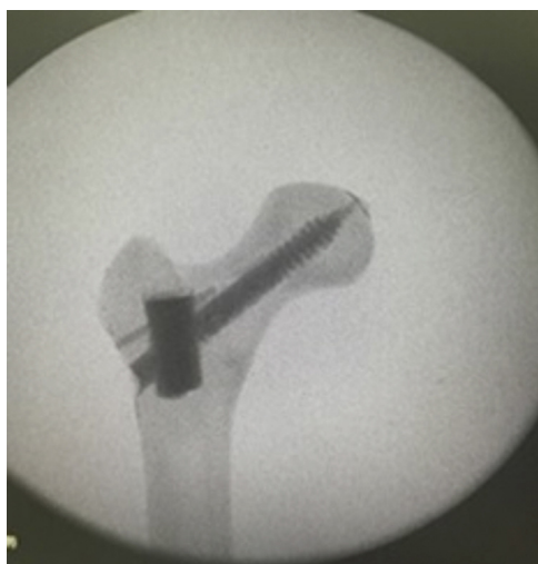
Fig. 2 – Radiographs of a synthetic model after PMMA reinforcement.
