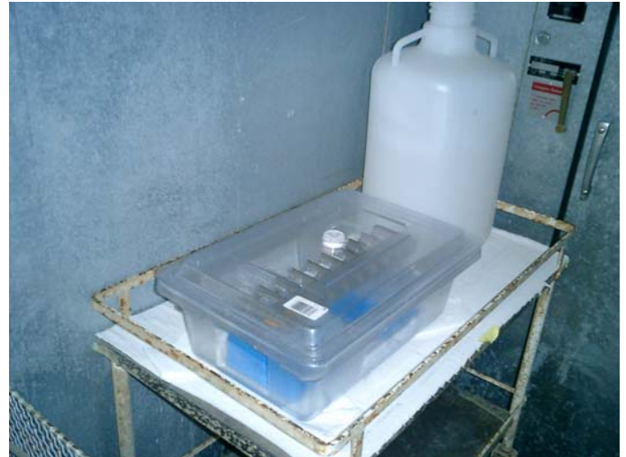
Fig. 2: For Immunofluorescence Immunohistochemistry (IF-IHC) procedure: Humidified chamber (containing the slides on the metal slide rack) being placed inside a cold room at 4°C. Notice the small leveling device atop the container to ensure that reagent run-off is not allowed.
