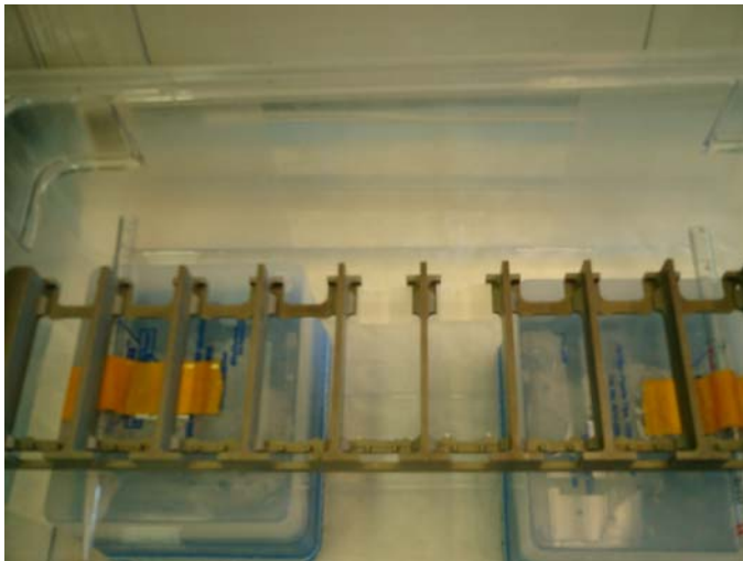
Fig. 1: 2 slides being stained by IF-IHC (preceding LCM) are shown in the middle of a metal slide rack within a larger, humidified and sealable container.
