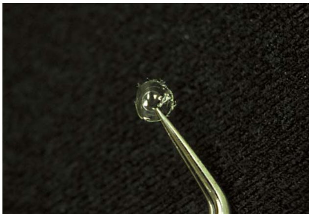
Fig. 21: The removed polymer tab; if desired, one can additionally trim the tabs closer to the central region where the captured cells are using a nuclease-free pair of scissors.
