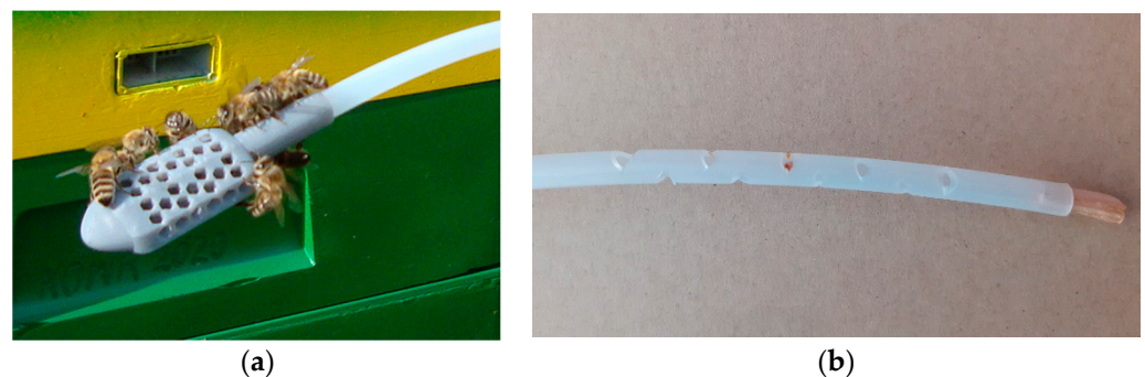
Figure 7. Sample probes used in our studies: (a) probe made in advance by 3D printing; the thickness of the probe is greater than the gas line diameter (6/4 mm); (b) probe invented and made in field conditions. The gas line was cut with small holes, close to its end. The probe has the diameter of the gas line.
