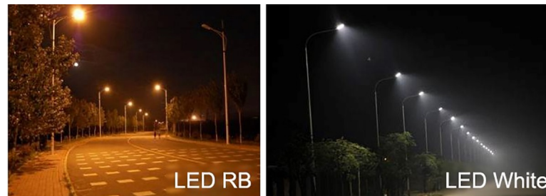
Fig 1. Appearance of lighting of red plus blue (RB) and white lights from streetlamps using light-emitting diode (LED) as source of lighting in Shenyang City, Liaoning Province, Northeast China.
