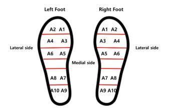
Figure 7. Sensor locations for plantar pressure detection.
