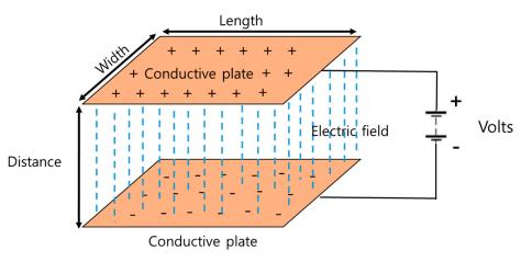
Figure 1. The structure of parallel capacitor used for the textile capacitive pressure sensing insole (TCPSI).
