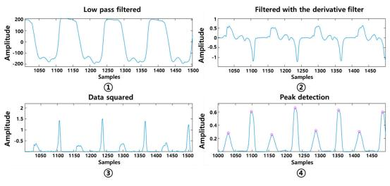
Figure 8. Signal processing order.
