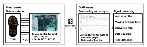
Figure 3. The schematic diagram of the gait monitoring system.
