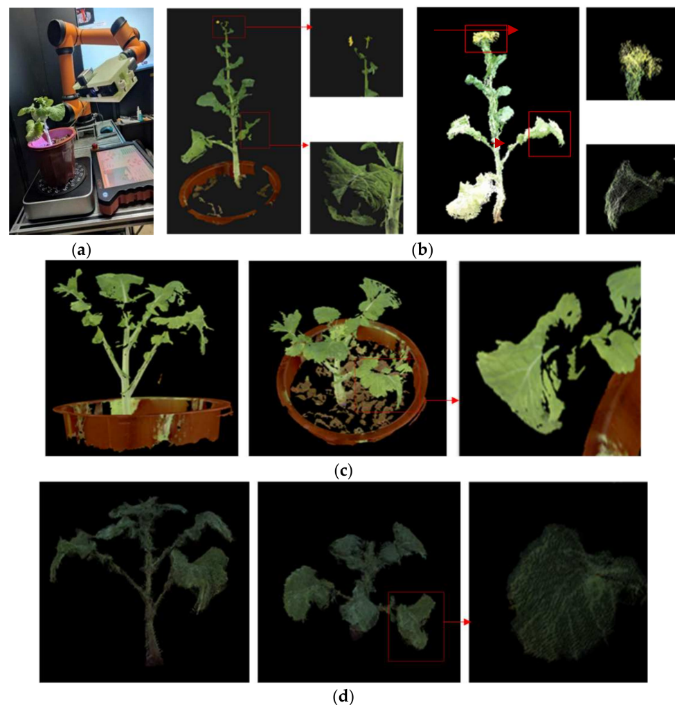
Figure 13. Comparison of the 3D reconstruction effect between the laser scanner and the algorithm in this paper. (a) 3D reconstruction of laser scanner (flowering rapeseed). (b) 3D reconstruction of our method using the same sample. (c) Another 3D Reconstruction of 3D laser scanner (Rapeseed in moss stage). (d) 3D reconstruction of our method using the same sample.
