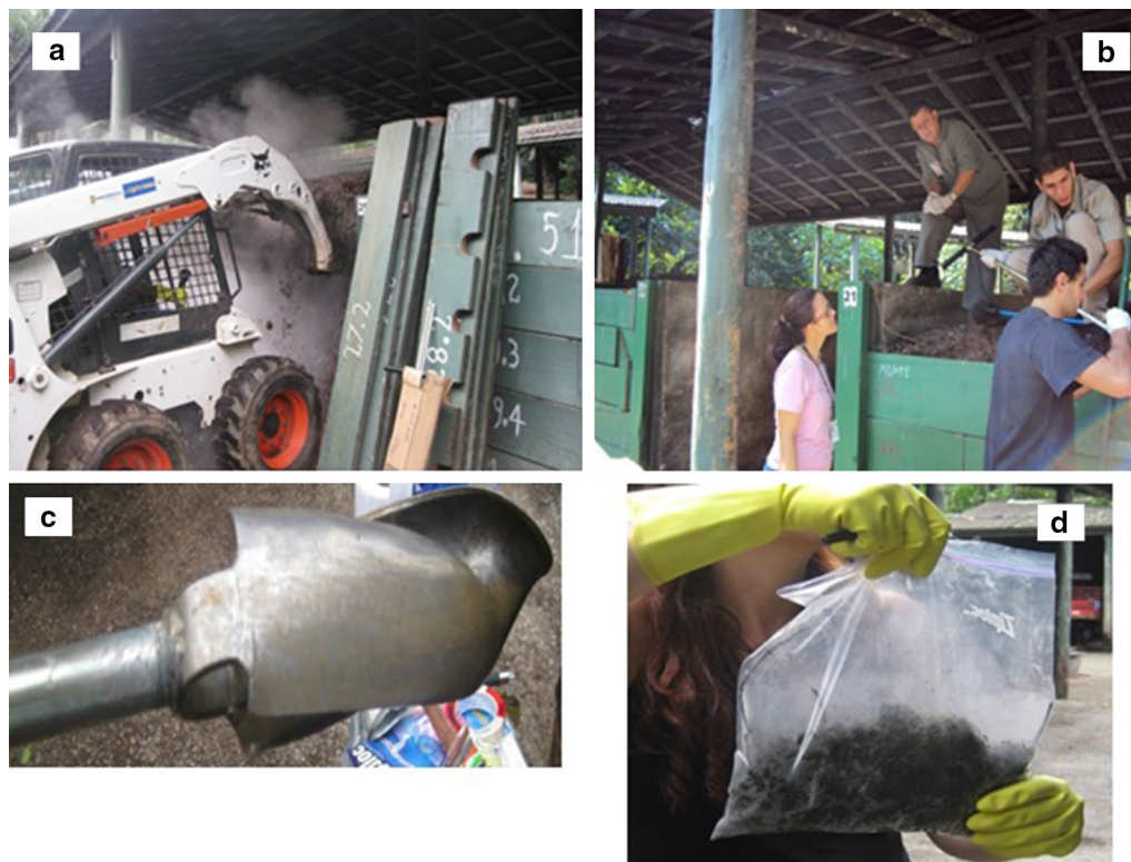
Fig. 1 a Illustration of the process to construct of a composting pile at São Paulo Zoo Park Foundation; b Illustration of technicians sampling material from the composting pile; c Adopted instrument that was applied to access all the layers that form the composting pile (Bitencourt et al. 2010); d Ready sample for microbiological analyzes
