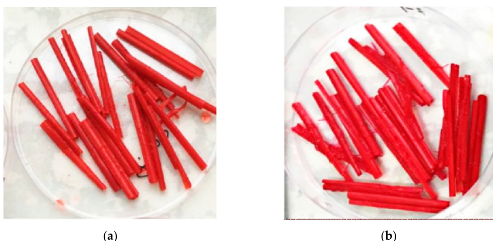
Figure 3. Dyeing effects Acid Red GR (a) and Reactive Brilliant Red X-3B on corn straw (b).
