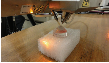
FIGURE 1: Spectrometric micro X-ray fluorescence ( \mu XRF). Bruker Model Spectra Artax (Berlin, Germany).
