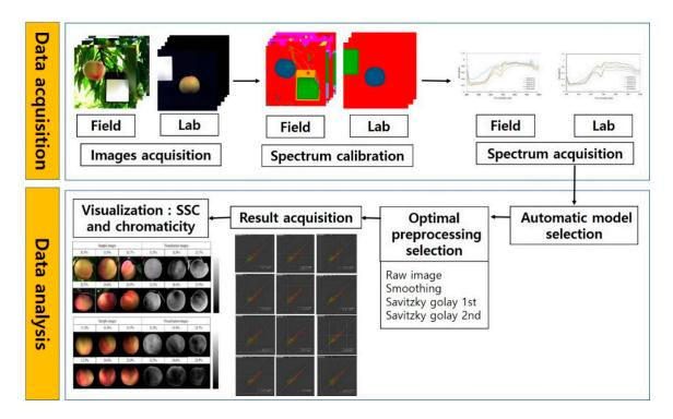
**Figure 4.** Flow chart of data processing procedures for prediction of physicochemical properties of 'Madoka' peaches based on lab- and field-based HSI applications.
