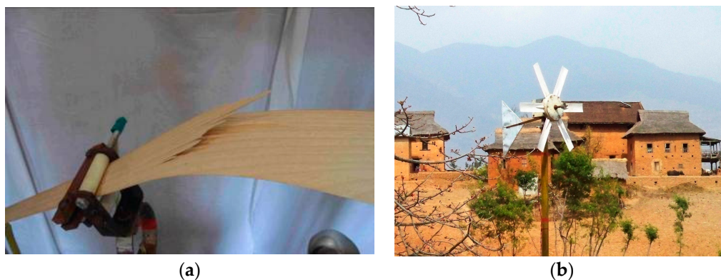
Figure 5. Testing the timber wind turbine blade (a) and small wind turbines installed in Nepal (b).
