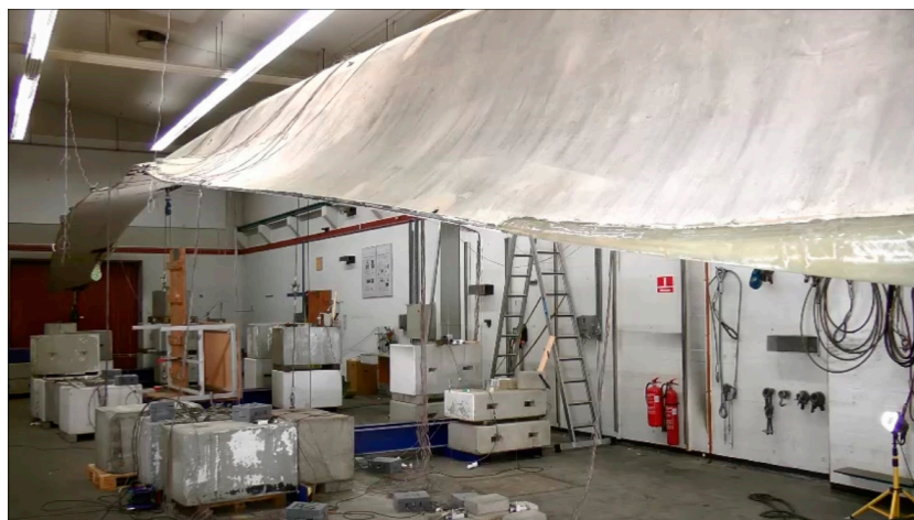
Figure 8. Full-scale testing: A 34 m long wind turbine blade subjected to static test in a combined flapwise and edgewise load direction.
