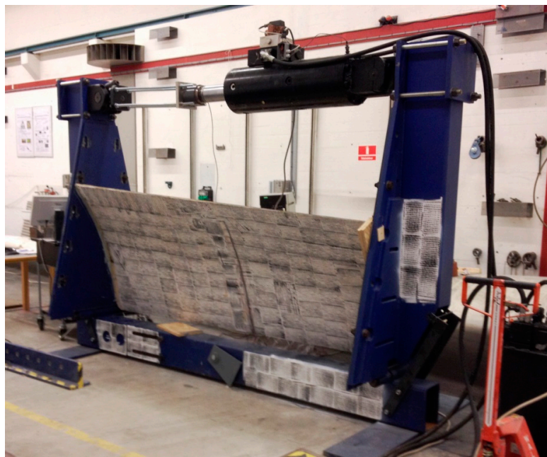
Figure 9. Sub-component testing of trailing edge panel in compression using the method developed at DTU.
