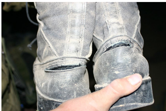
Fig. 1 Damage to the heel counter of the HWIB
