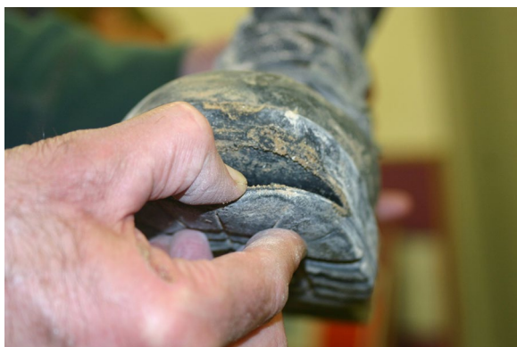
Fig. 2 Delamination between the outer rubber and inner polyurethane layers of the HWIB sole
