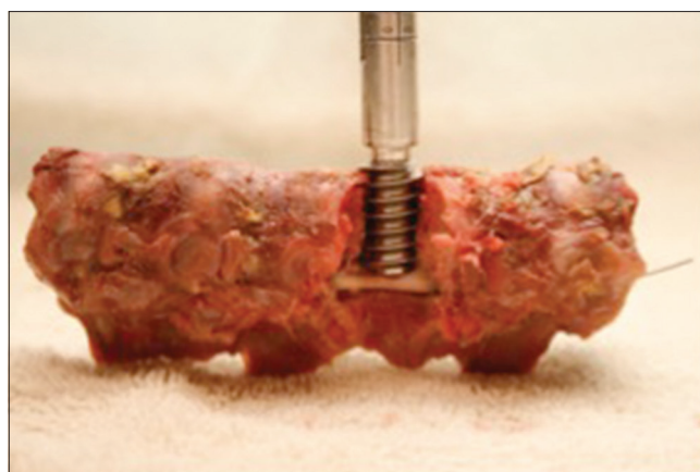
Figure 1: Example of the experimental setup. Each spinal segment underwent graded spinal canal compromise with the use of a modified 12.7 mm dynamic hip screw. Part of the vertebral body has been removed for demonstrative purpose
