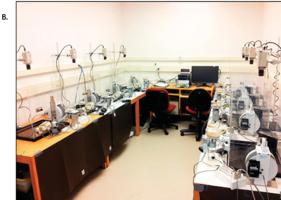
Figure 2. Integrated Behavioral Station. (A) Schematic representation of hardware, and software used in designing an INBEST box (L = 39 x W = 53 x H = 50 cm). (B) Eight complete INBEST boxes provide an opportunity for concurrent home-cage monitoring of four experimental and four control mice.
