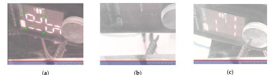
**Figure 4.** Possible states of the oximeter display. (**a**) Complete reading procedure and points (in green) needed for the oximeter image alignment; (**b**) oximeter turned off; (**c**) incomplete reading procedure.
