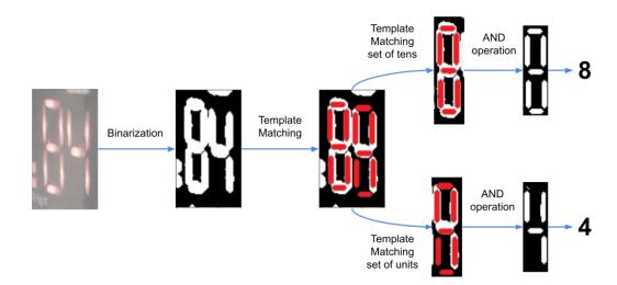
**Figure 7.** Diagram of the OCR recognition algorithm using the aligned image (the oximeter display in this example) to search for key pixels applying template matching and return the displayed value in text format.
