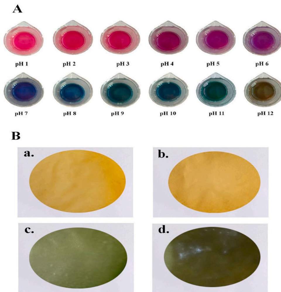
Fig. 2. (A) Colour variations of CTE solution, (B) physical appearance of a) SPI, b) SPI-CNW, c) SPI-CTE and d) SPI-CNW-CTE films. (For interpretation of the references to colour in this figure legend, the reader is referred to the Web version of this article.)
