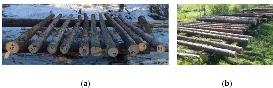
Figure 10. Single-stem set-up of storage experiment in winter (a) and summer (b) in 2017.
