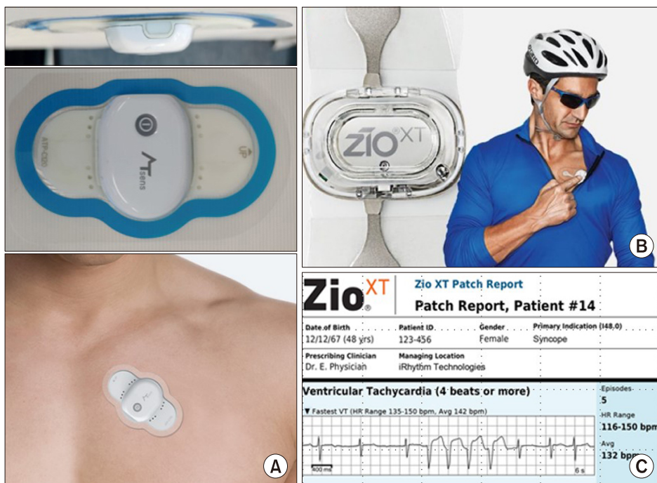
FIG. 2. Examples of patch type single lead ECG recording devices. ATP100 (ATsens, Seongnam, Korea) (A), Zio Patch (iRhythm Technologies, San Francisco, CA, USA) (B), ECG recording from Zio patch (C).
