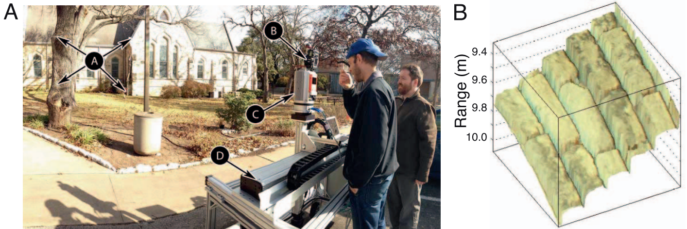
Figure 2. Registered range and camera images. (A) Camera and laser range scanner mounted on portable four-axis robotic gantry: (A) natural scene, (B) Nikon D700 DSLR camera, (C) Riegl VZ-400 3D range scanner, (D) custom robotic gantry. (B) A 200 \times 200 pixel patch of a camera image of stone structure mapped onto the range image. The registration is generally within plus or minus one pixel. Note that the shadows in the camera image coincide with the mortared seams in the stone structure.
