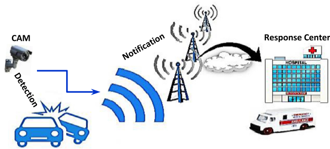
Fig. 1. Automatic vehicular accident detection and notification.
