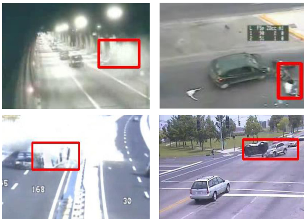
Fig. 7. Sample snapshots from some video clips for vehicular accidents correctly detected by the presented system.
