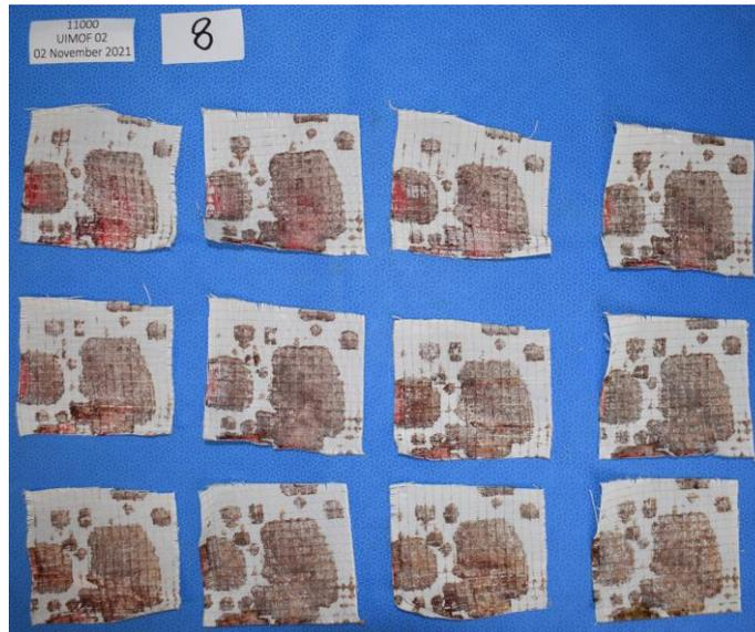
**Figure 5. Layout example of membrane gas transfer fiber sheets for digital imaging**
