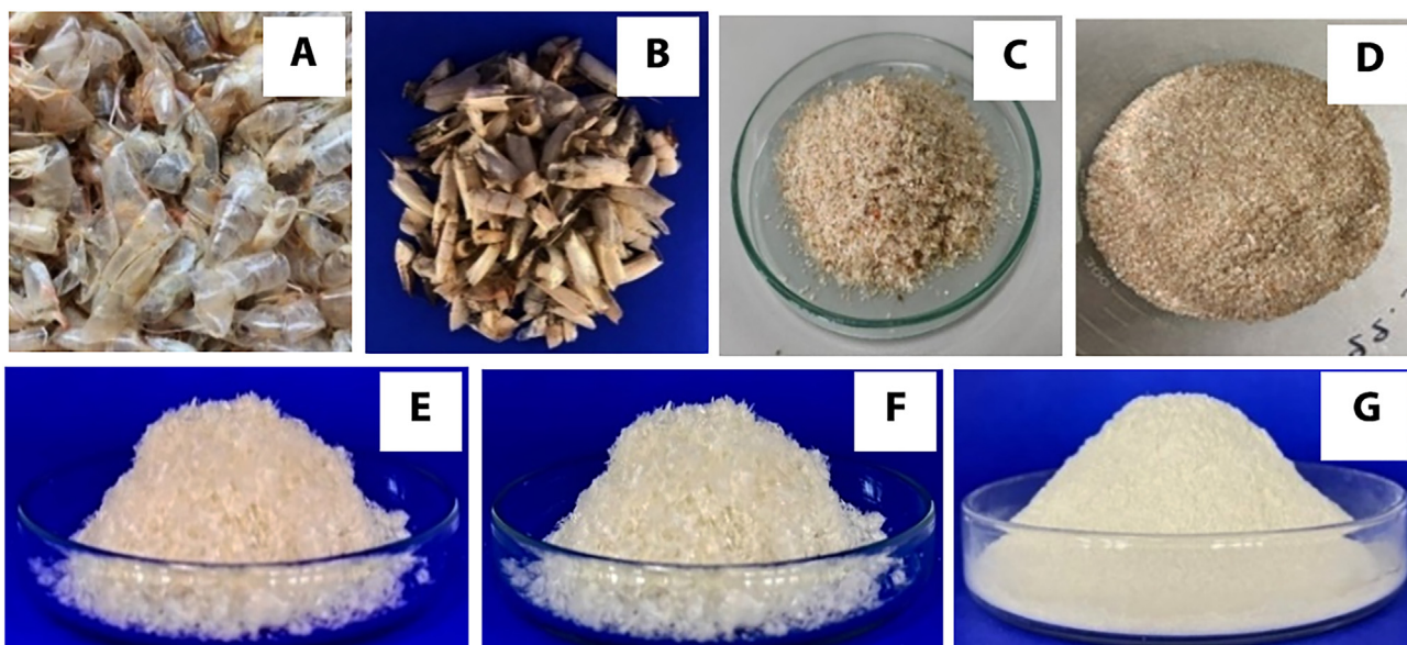
Figure 5. Physical characteristics of (A) shrimp shell, (B) dried shrimp shell, (C) shrimp shell powder, (D) shrimp shell powder demineralization, (E) chitin, (F) chitin decolorization and (G) chitosan (CS).
