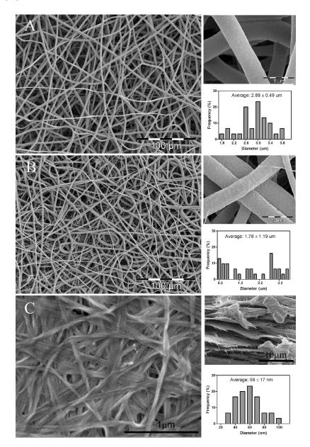
**Figure 1.** SEM images and fiber diameter distribution of nanofibers. (**A**) PLA from 8 wt % PLA in chloroform/acetone (3:1, v/v) solution; (**B**) PLA/Lip from 8 wt % PLA in chloroform/acetone (3:1, v/v) containing 5% lipids (PLA w/w); (**C**) BC sample surface.
