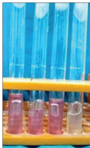
Figure 4: Sugar fermentation test (positive for Candida tropicalis and C. kefyr )
