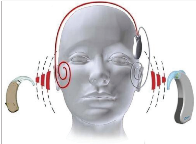
Figure 11. Schematic representation showing sounds acquired by the microphone of a conventional speech processor and by the contralateral microphone connected to it. Both are processed by the speech processor and sent to one single implanted receiver-stimulator, responsible for transmitting the information simultaneously to the ipsilateral and contralateral electrode beams, so they synchronously stimulate the neural fibers of both cochleas.
