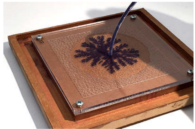
Figure 1. Hele-Shaw experimental setup performing a Viscous Fingering experiment. Adapted from Salmaan Craig [1].
