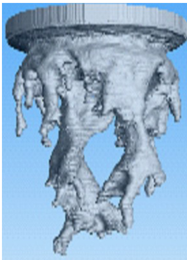
Figure 7. Experimental results of 3D VF in a cylindrical packed bed. The results were obtained with a micro-focused x-ray tomography scanner. Image adapted from Suekane [22].
