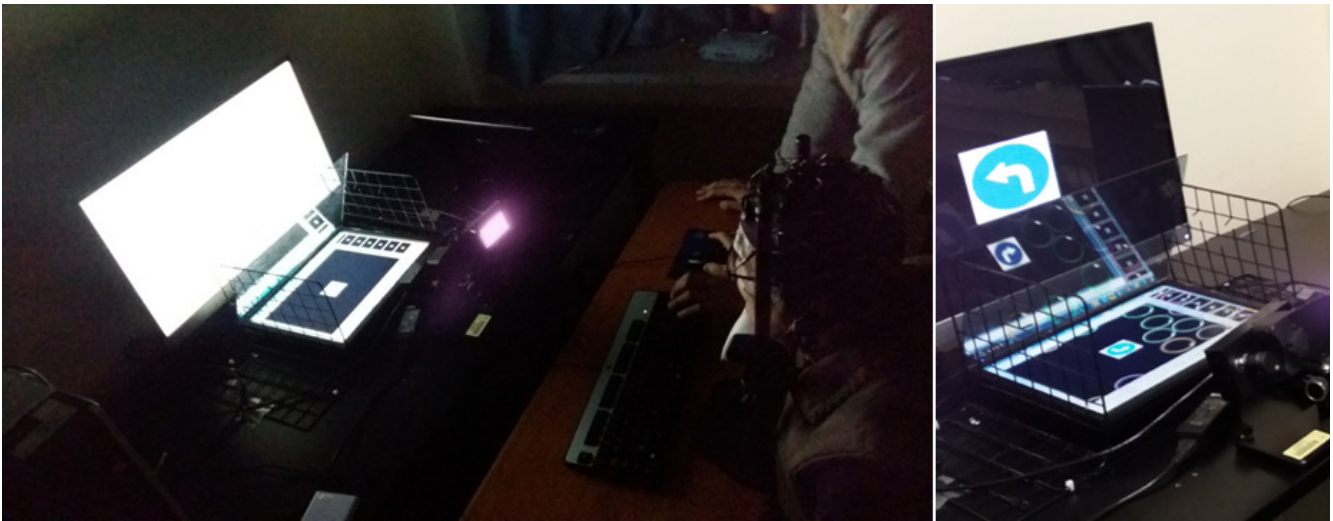
Figure 2. HUD display device constructed in the laboratory: Instead of the HUD device in the vehicle, a reflector was made with a simple fixing device with a glass plate, and the position of the face was adjusted and fixed for each individual so that two traffic signals could be clearly seen.
