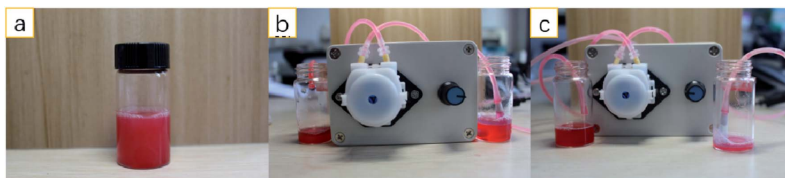
Fig. 13 Process diagram of oil–water separation test in emulsified state ((a) the initial emulsified mixture of oil and water as prepared, (b) the separation process of the emulsified mixture, and (c) the finishment of the separation process of the emulsified mixture).
